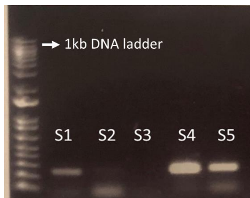
Figure 7. 1% agarose gel image of different PCR controls in VCSEL-based plasmonic and conventional thermocyclers.
